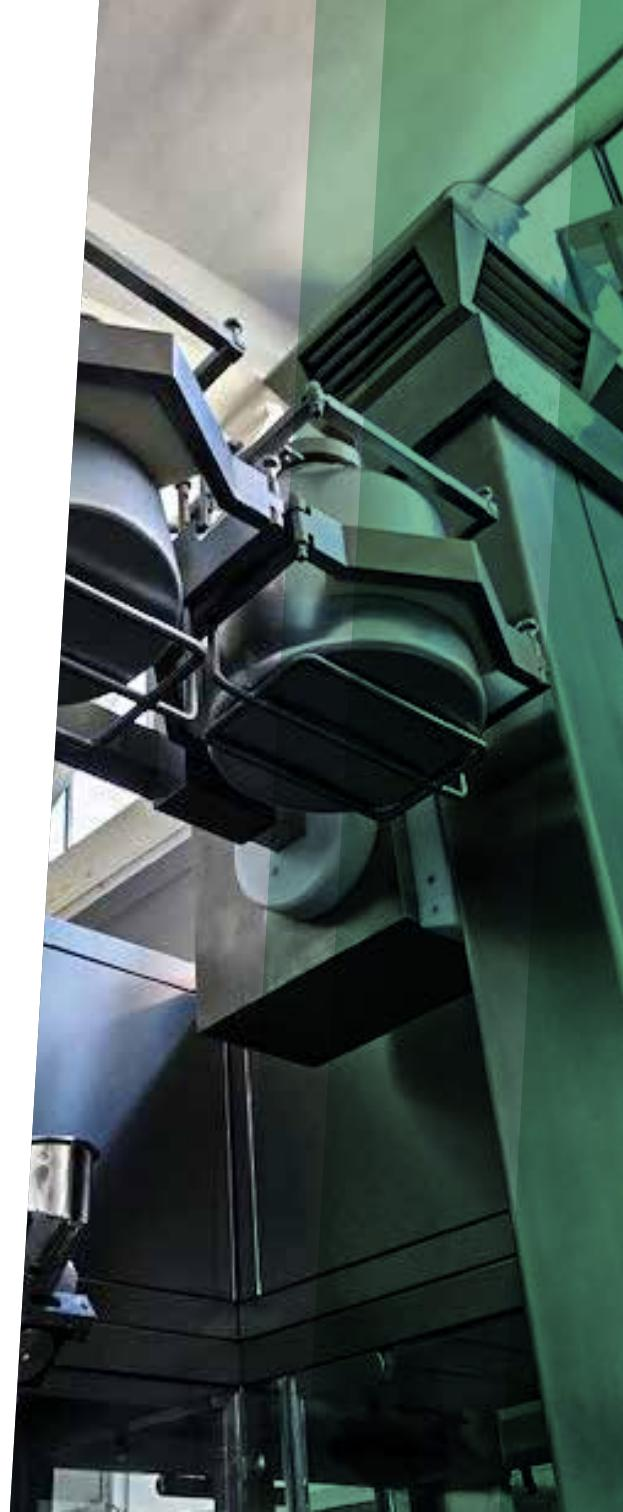
The **lifting column PHARMA LIFT**, is the machine with the **highest level of customizations** produced by Bimech Srl. PHARMA LIFT is designed for handling several containers or machineries in pharmaceutical, chemical and food Industries. The machine can easily and safely lift a container to the suitable height for the requested function.
