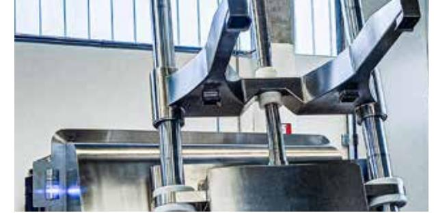
The bins are placed in the cradle of the structure by the operator, and the machine will move the lower platform bringing the container to the mixing start position.
