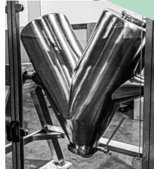
This category of mixers differ from the previous one essentially due to the fact that the tank containing the powders is an integral part of the machine and is not removed for loading/unloading and cleaning.
